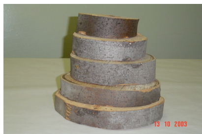
Figure 2 : The disks from which the specimens were cut
